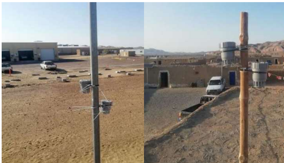
Diffusion tubes installed at RDMS
