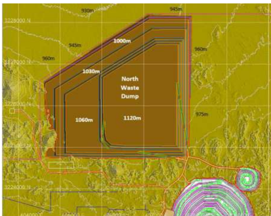
Figure 3-19: North Waste Dump Design
